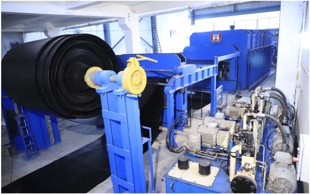
HYDRAULIC HOT PRESS CURING RUBBER CONVEYOR BELT
